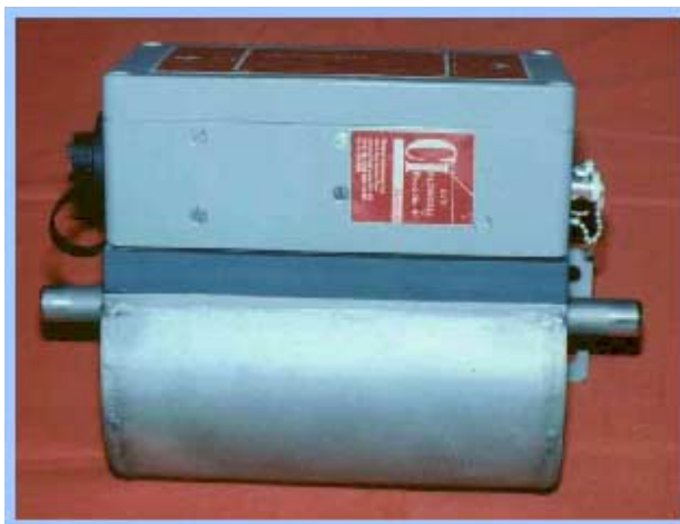
Figure 2: The CT Flowcell, operated on UK fisheries vessels
