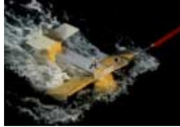
SeaSoar is the world's leading open ocean towed undulating data acquisition vehicle.
